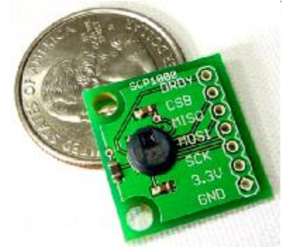
An absolute pressure sensor that uses MEMS technology
